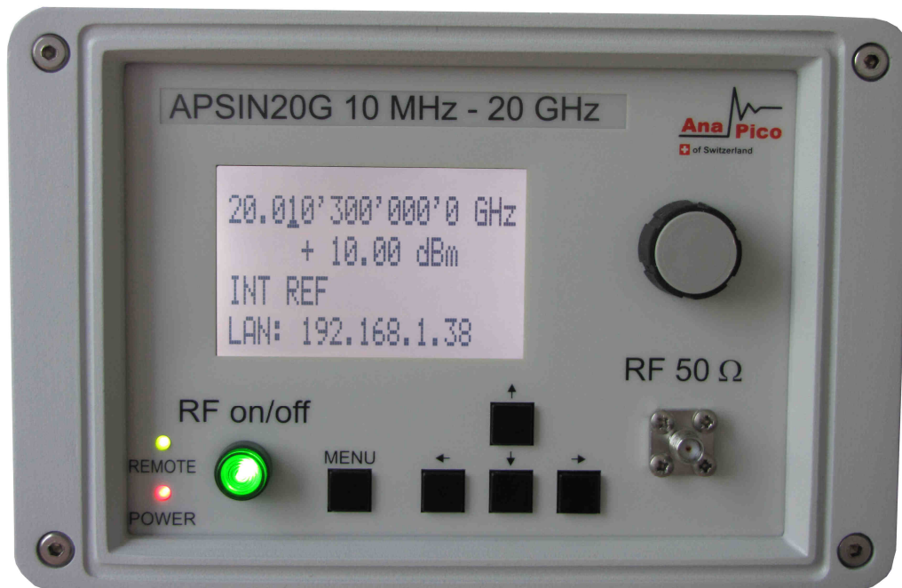
Figure 1-a APSIN Front Panel View (Model APSIN20G)
